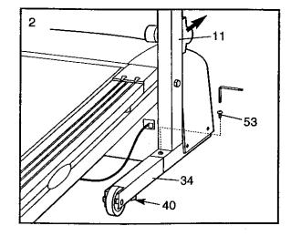
3. Remove the Handrail Screw (53) from one of the Handrails (1). Insert the Handrail into the tube at the top of the left Upright (11), and align the hole in the Handrail with the slotted hole in the Upright. Loosely thread the Handrail Screw into the Handrail, rotate the Handrail until the Screw is touching one end of the slotted hole, and then fully tighten the Screw.
